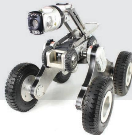
For heavily silted pipes we recommend the optional 250mm Balloon Wheel (QRW250/140/150), which are also required to centralise the crawler in 1000mm pipes.
